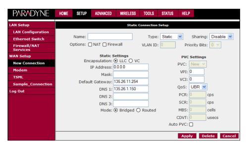
Figure 3-9. Static IP Connection Setup
